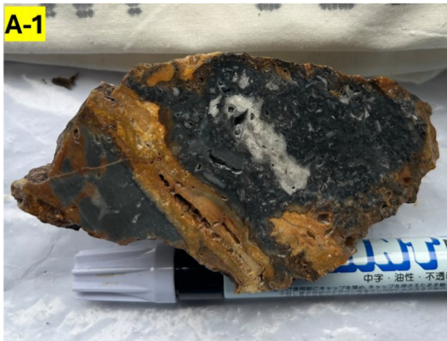
Figure 4 Representative rock samples and old mining tunnel photos from the Shika Prospecting Right. Float sample NT-0665 collected at the Unoya historical mine waste dump site, a 10 cm wide gray/ white weakly banded quartz vein with drusy center accompanied by silica and fine-grained sulfides (A-1), float sample NT-0485 collected at the Unoya historical mine waste dump site, a 30 cm by 10 cm angular white quartz vein about 3-6 cm in thickness, open-spaced cavities, partially brecciated with crustiform (colloform-cockade textures).
