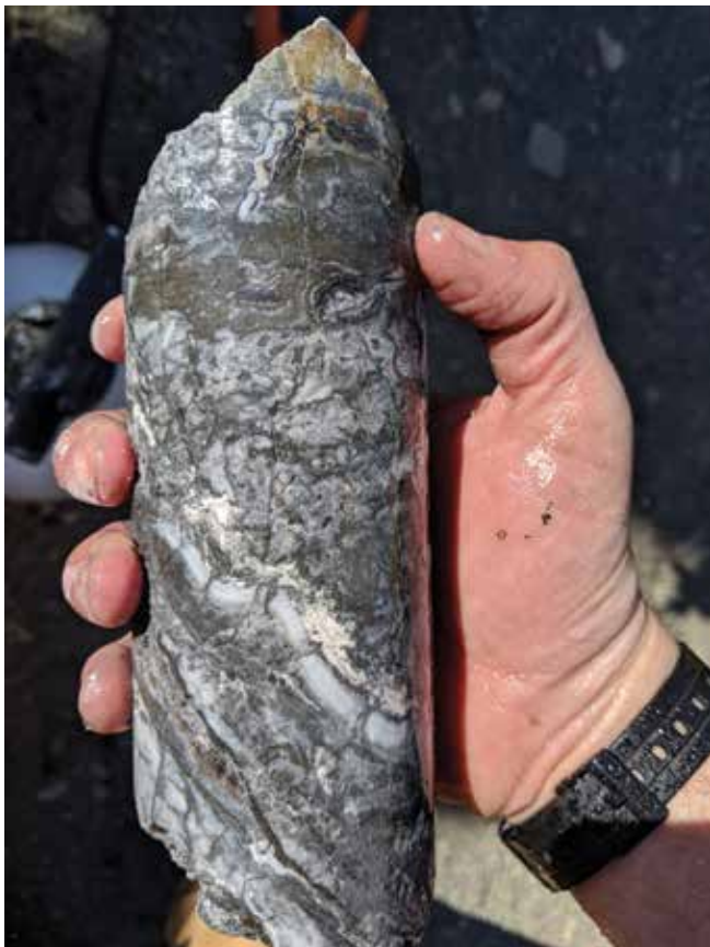
Diamond drill core showing banded quartz-sulfide vein from approximately 85 metres in hole 19OMS-002. Photo courtesy Irving Resources Inc.
